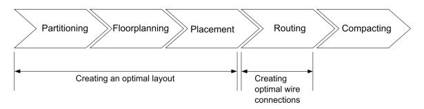
Figure 2: Basic process to create a microchip design
